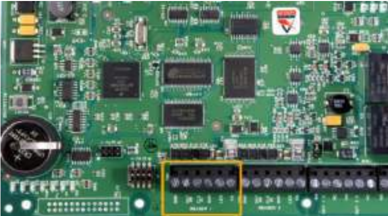
Figure 2: Mercury EP1502 controller boards
