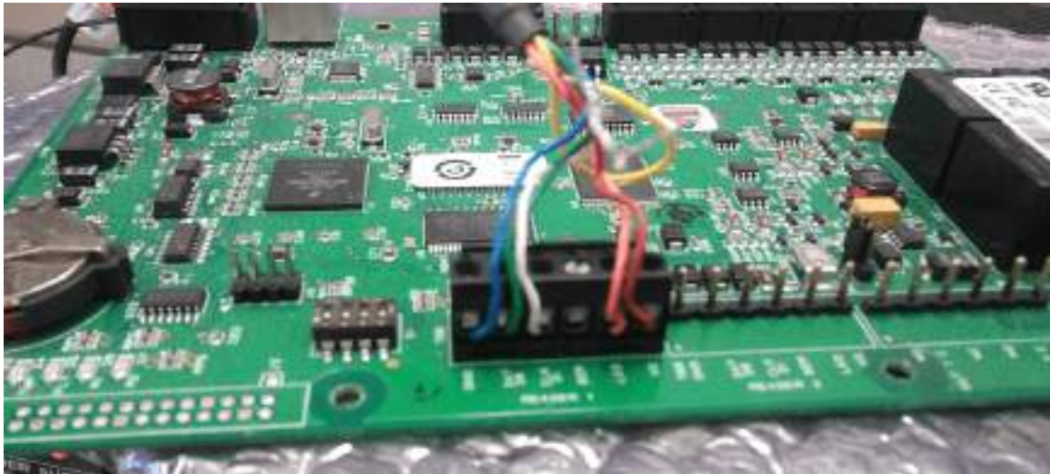
Figure 3: Mercury EP1502 controller board wiring loom connections
